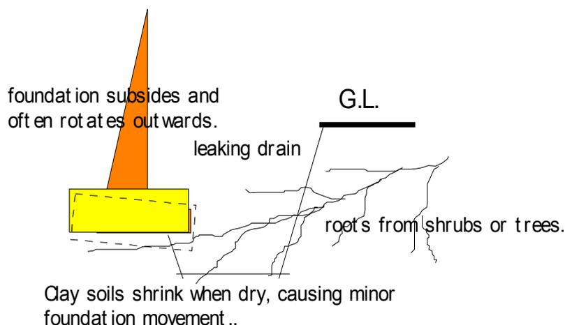
How roots infiltrate into the clay soil beneath foundations and the resulting damage - outward rotation of the wall.
