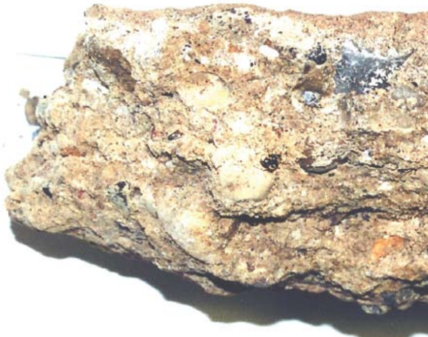
(c) 70 mm thick sample of oversite concrete affected by TSA. The concrete has been softened and discoloured white and yellow-brown. Much white thaumasite can be seen in the upper part of the section. Concrete missing from the bottom of the section was so friable it fell away during sampling.
