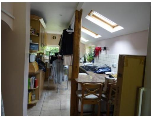
The walls and ceilings are plastered, finished with emulsion. Slight board cracking was noted to the underside of the skylights which is of no structural concern and requires filling prior to decoration.
